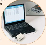
Because the SCS triggers termination of the compaction effort, SCS testing is completed before end result testing can even begin. Because the SCS controls the compaction process and brings each lift to maximum achievable stiffness and corresponding density, rework is virtually eliminated. Conversely, end result testing does not control the pre-test compaction process, is comparatively slow, does not detect protocol violation and often results in rework and/or pavement failure.
