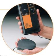
process. The SCS determines when continuing compaction activity has reached a point of diminished returns relative to increasing wave amplitude, i.e., has ceased providing meaningful improvement in soil stiffness (force/deflection). At that point, the SCS gives a visual signal to terminate compaction activity and documents whether or not its instructions were followed. The SCS monitors, manages, and documents performance relative to the compaction effort.
